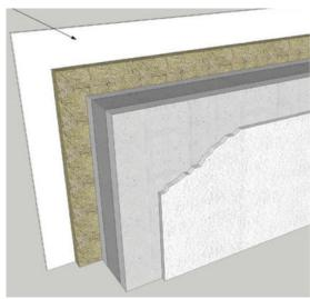
Inside Walls the partitions walls of the housing units will be of internal metal structure, internal acoustic insulation and plasterboards (Pladur type)
